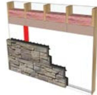
Standard framed wall with OSB or plywood
